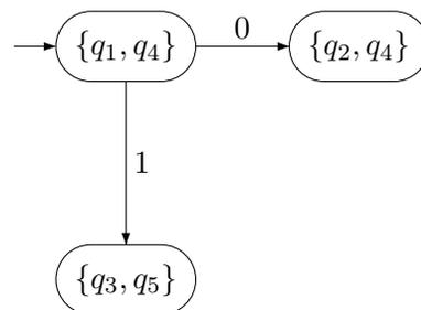
Let us repeat the process for another transition. To illustrate the process of simplifying, suppose we look at the transition leading from the state  $\{q_2, q_4\}$  labeled by 1. We would obtain this diagram:
